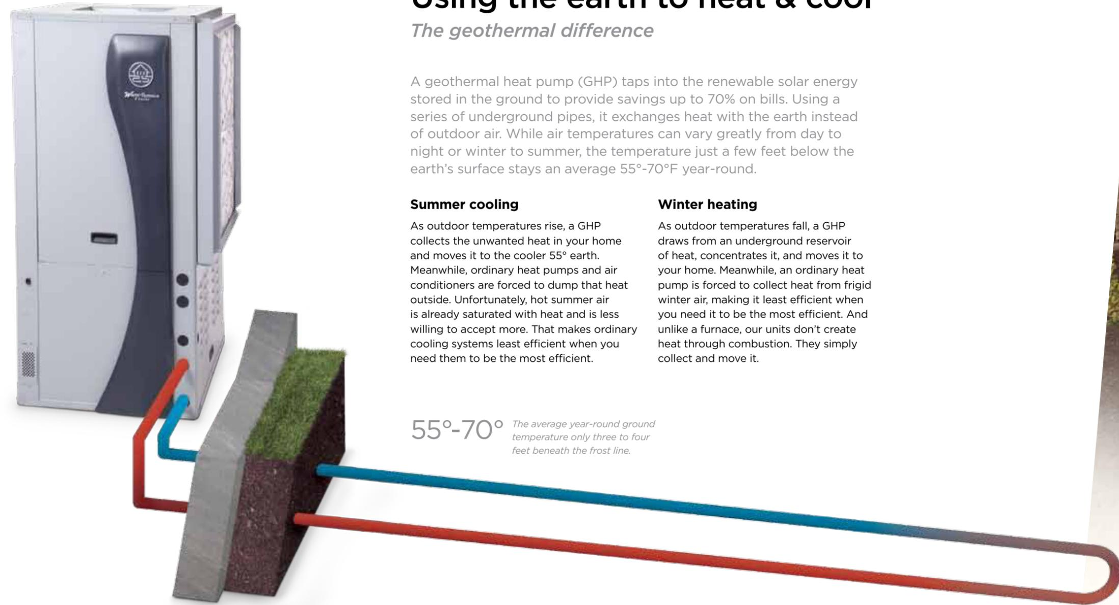
Note: Illustration represents how geothermal works and is not to scale. Loops are generally 4-6 feet below the earth's surface and between 150-400 feet long.
